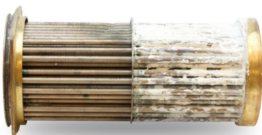
After cleaning (left) and before cleaning (right).
