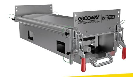
The PureBelt® Fixed Systems are designed for cleaning flat belts (webs) in a wide range of environments, from dry environments where wet cleaning has to be avoided, to damp and wet environments. The systems use steam to break down debris and oils, sanitizing as it works. An efficient vacuum draws away the debris and moisture to leave the belt dry. An optional motorized brush is also available.
