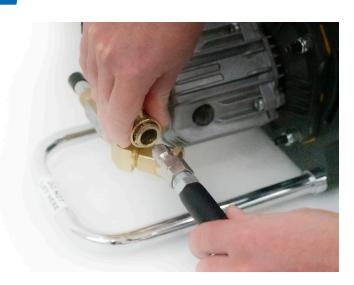
Attach the spray gun to the quick connect of the high-pressure hose.
