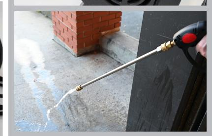
Attach either the black nozzle or wonder-wand to the spray gun's quick connect to siphon and apply soap.
