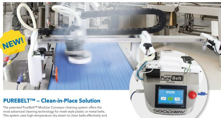
safely, conserving 90% more water than other cleaning methods. Using the innovative spinning steam head, conveyor belts are quickly cleaned of soils, sugars, fats, and allergens, leaving belts ready for immediate production. You can use the system across multiple belts in your facility, and it can be sized to fit your exact conveyor dimensions.
