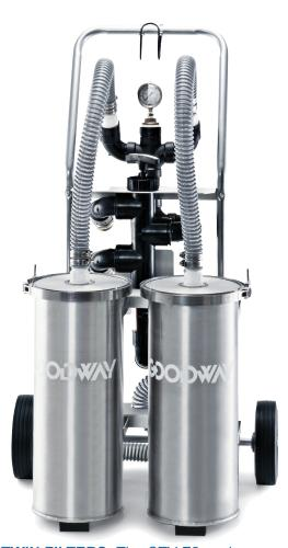
TWIN FILTERS: The CTV-F2 works in tandem with Goodway's TowerVac to filter and return cooling water to the basin. Its reusable filter cartridges scrub cooling tower water down to 5 microns and recirculates it at up to 50 gallons per minute.
